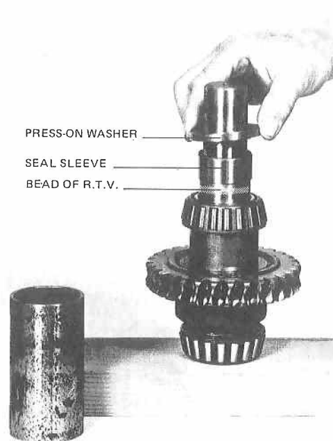
Figure 2 SEAL SLEEVE INSTALLATION
